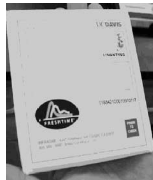
Pilot trials of temperature and vase life monitoring using active RFID chips were carried out with these prototype CD-sized tags.
